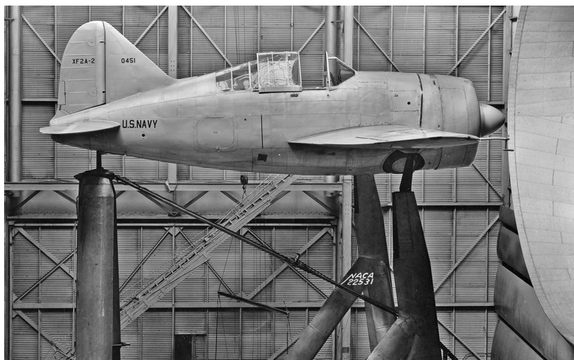
Fig. 12 XF2A-2 mounted on the Langley full-scale wind tunnel for drag-reduction studies following the flight compressibility project. (Photo courtesy NASA Langley Archives via Susan Seward.)
